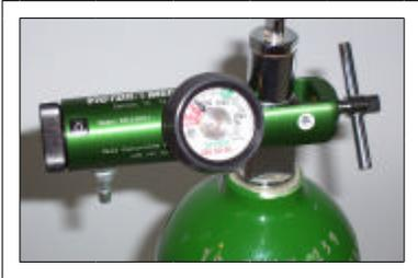
I started with the decision to use the Oxymizer® mask. It's claim is to use 75% less oxygen on average. Therefore, I needed a regulator capable of supplying .25 to 1.0 liters per minute flow rate. If I wanted to share the system with two people, the flow rate had to be between .25 and 2.0 liters per minute. I chose the SlimLite II pediatric regulator made by Victor Medical (victor part #07813323). See web url:
