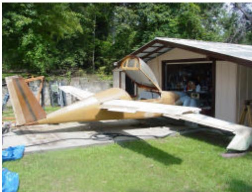
2<sup>nd</sup> project is a standard Dragonfly built from plans. Fuselage sides & belly pan and bulkheads done, wing completed, and all foam for rest of plane is cut ready to glass, all glass to finish and carbon fiber included, nearly complete Ken Brock metal control kits, Fiberglass hoop gear, wheel and tires, brakes, + more,
