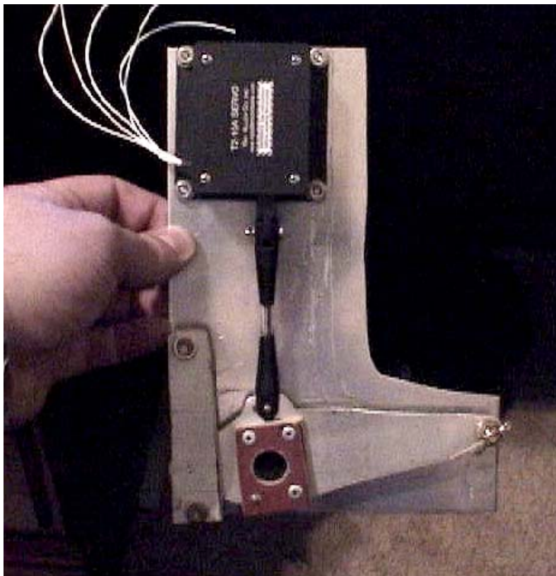
Figure 7: Completed reflexor ready to bolt onto bulkhead.
