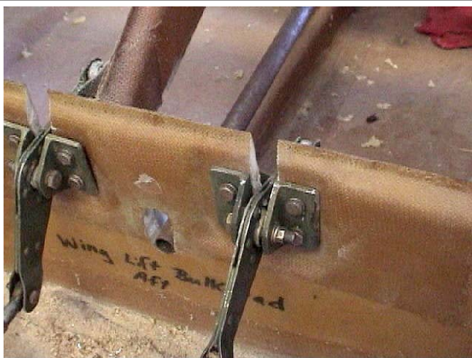
Figure 1: Area on the Wing Lift Bulkhead where the reflexor will be mounted between the motion changers (looking forward)
