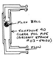
fittings so the ball could not be pushed up against the fitting and restrict the flow. I then mounted the indicator in the instrument panel (with the soldered wire at the top of course) and plumbed the fuel pump to the bottom and header tank fill line to the top - works great!
