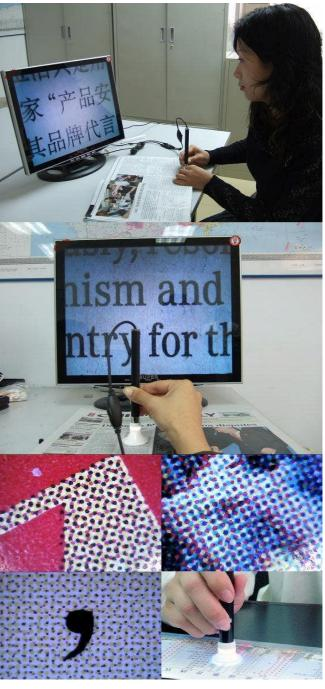
a focusing cap is that it saves you from the need to constantly adjust the focus when you use the pen camera to view flat surface materials and have to constantly move the camera. By attaching a focusing cap to the pen camera, you can press the cap against the surface of the materials you want to view and thus always maintain a constant distance between the lens of the pen camera and the materials.
