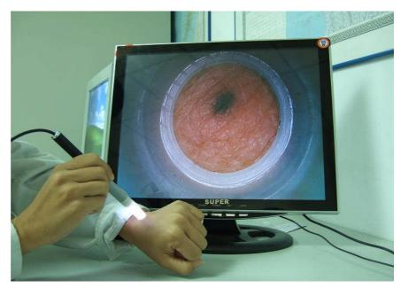
advantage of using a multi-function tube is that it saves you from the need to constantly adjust the focus when you use the pen camera to view parts or flat surface materials and have to constantly move the camera. By attaching multi-function tube to the pen camera, you can press the tube against the surface of the materials you want to view and thus always maintain constant distance а between the lens of the pen camera and the materials.
