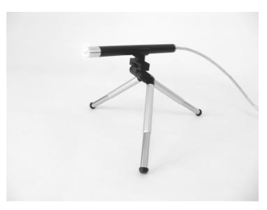
Since the focus of the lens is at the edge of the front-end opening, you can see virtually anything you point at. At the same time you still can adjust the clarity of the image by rotating the focusing ring while viewing.
