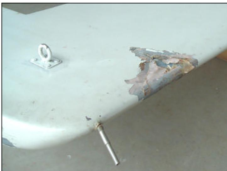
*Here is the underside of Mark's canard showing the damage from the impact with the sign—ouch.*
