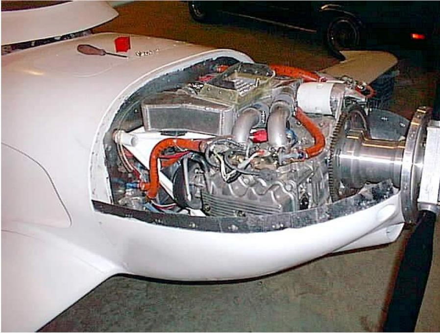
We removed all accessories, intake, and hoses, and the bell housing was cut off.
