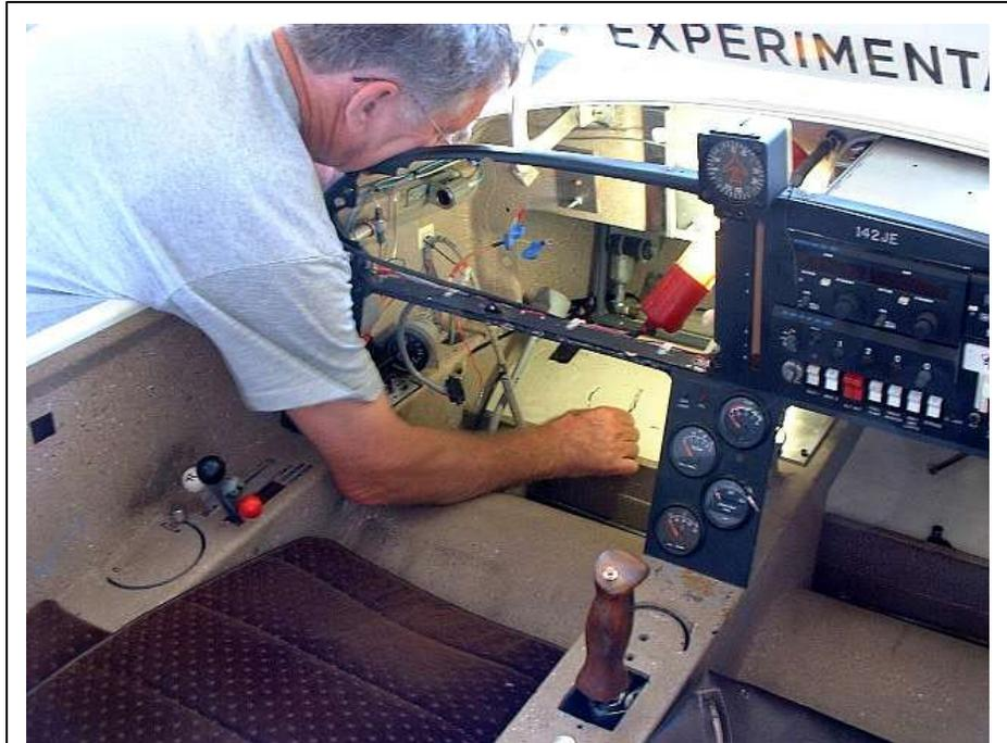
**John Mason defining the damaged area with a coin and a marker**
