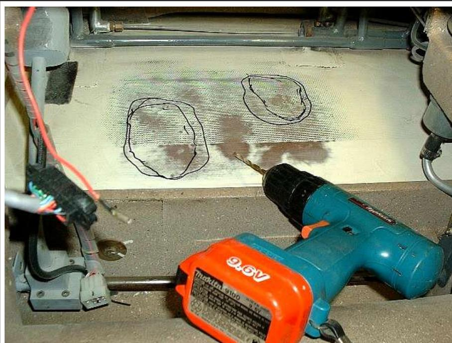
**Paint removed, holes drilled, it's time to inject micro!**
