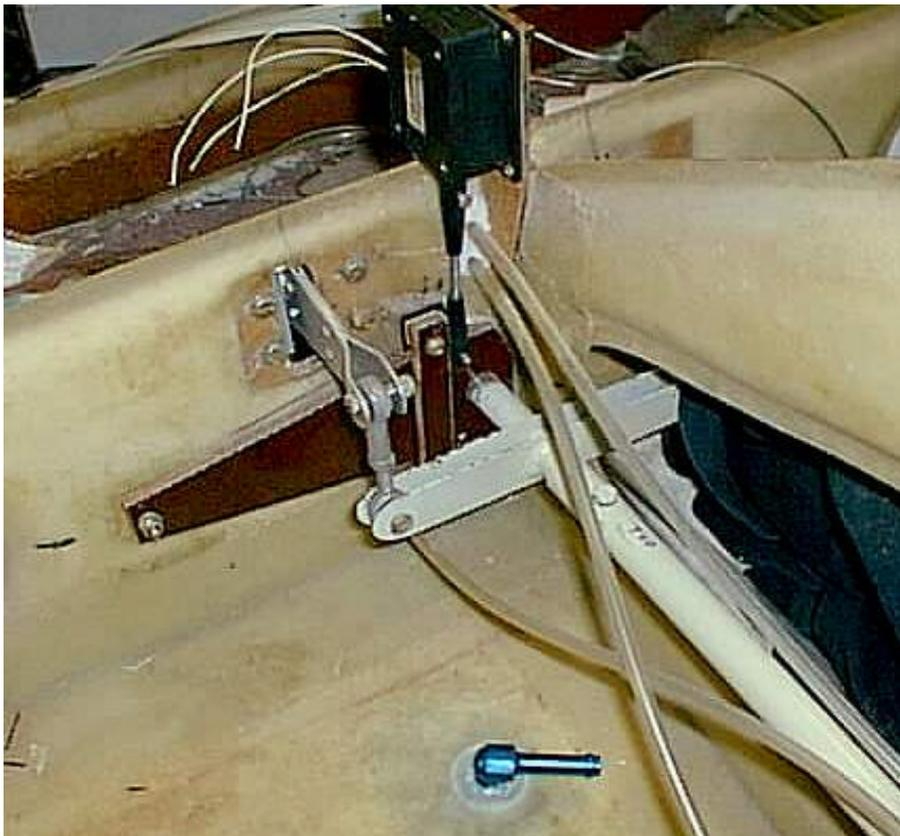
**Check this photo closely. It's a very simple and elegant electrically actuated reflexor mechanism.**
