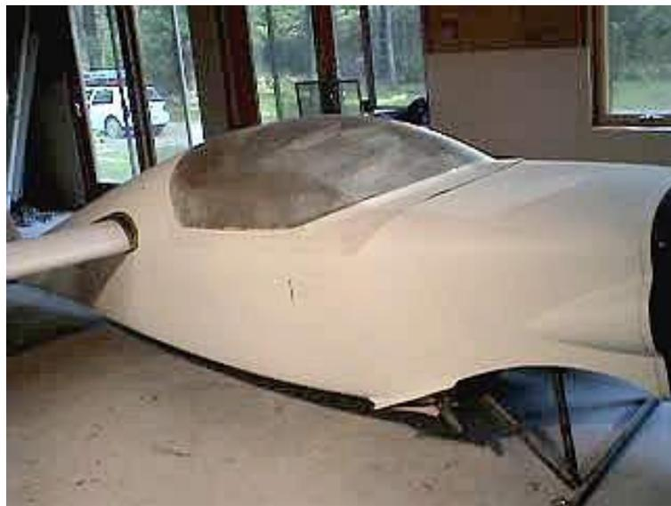
Right side, showing the canard root fairing, and part of the "rolling fuselage" fixture.
