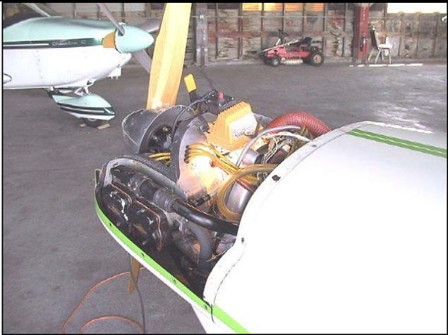
**One of the two cracked engine cases is warmed by a high power light for the proper curing of the soon to be applied JB Weld.**
