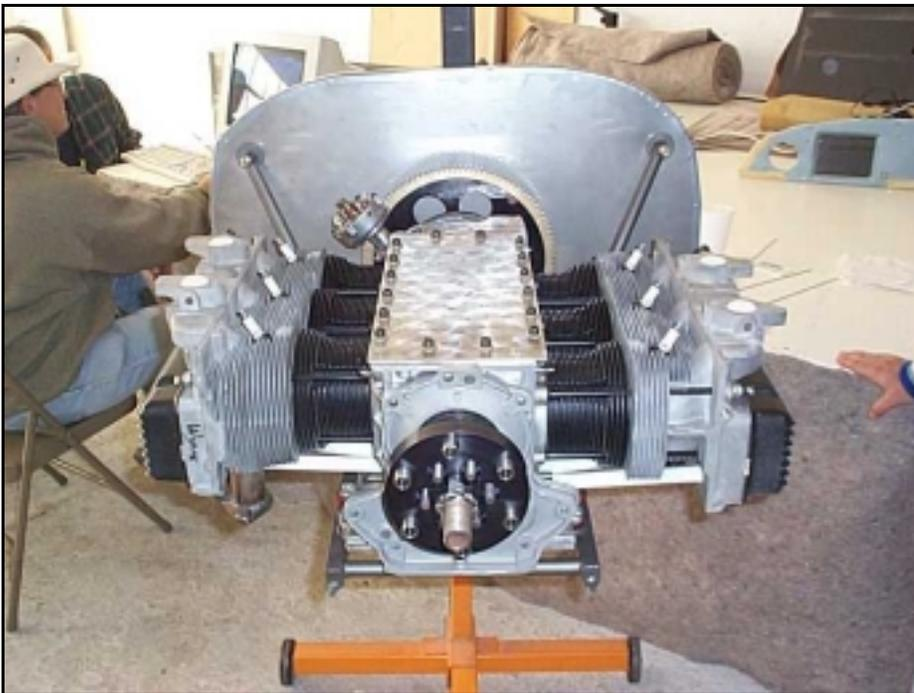
**William Wynne's 3100cc 6 cylinder Corvair engine. In smaller trim (2700cc) this engine produces a reliable, honest 100 hp @ 3200 rpm, and weighs in at under 250 lbs all up. This actual engine is highly experimental. It will be turbocharged, and should make 140hp or better, at altitude.**
