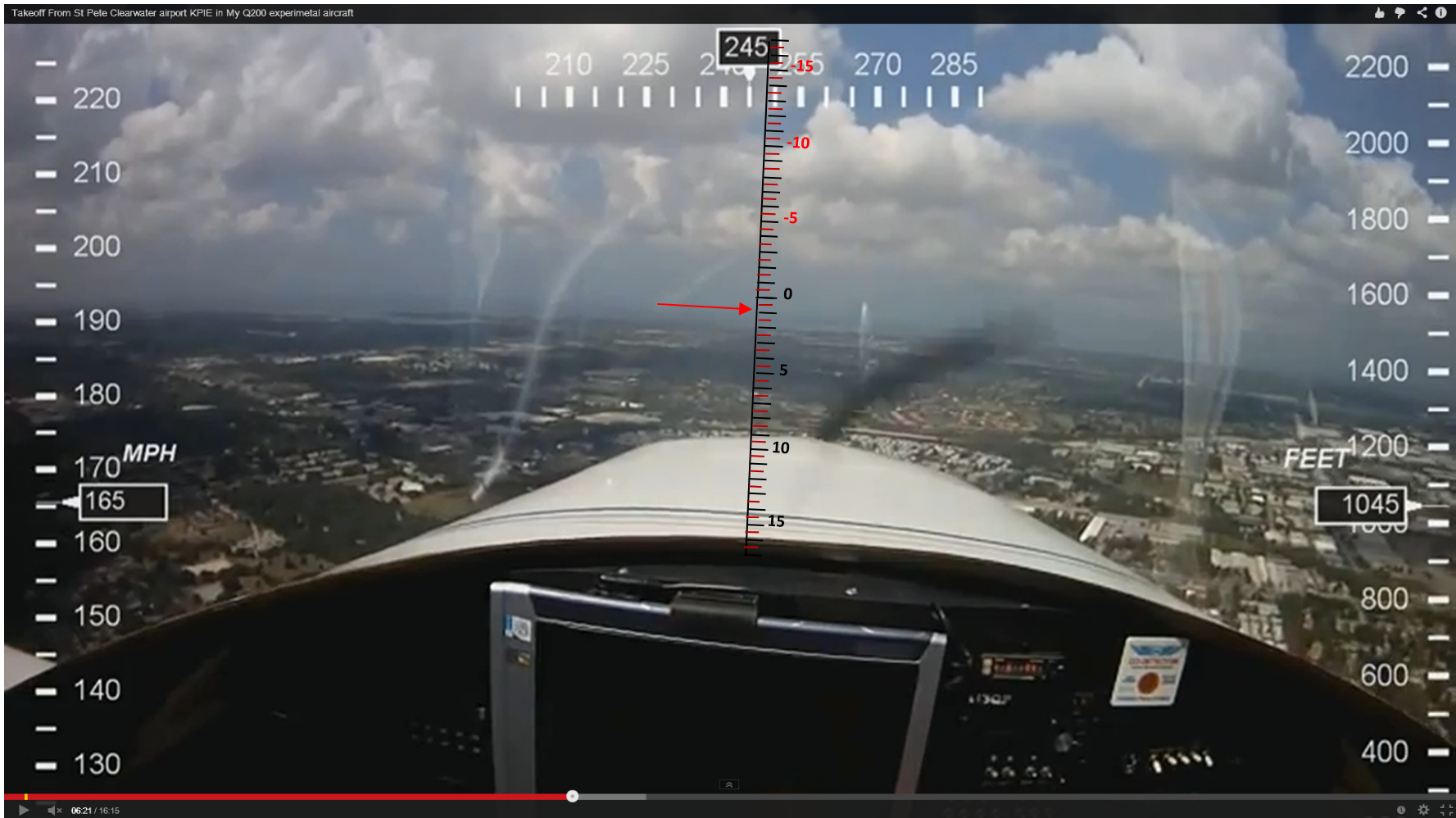
Figure 11. View from camera mounted on the seatback bulkhead. The vertical scale in the middle of the image is an angular scale that is calibrated to fixed points on the aircraft. The other scales (from Dashware) are: altitude (right), speed (left), and heading (top). This view is level, over 1000 feet MSL altitude and approaching max cruise (165 mph) at an alpha of 0.9 degrees. No confirmation of elevator deflection is possible at this point in flight.
