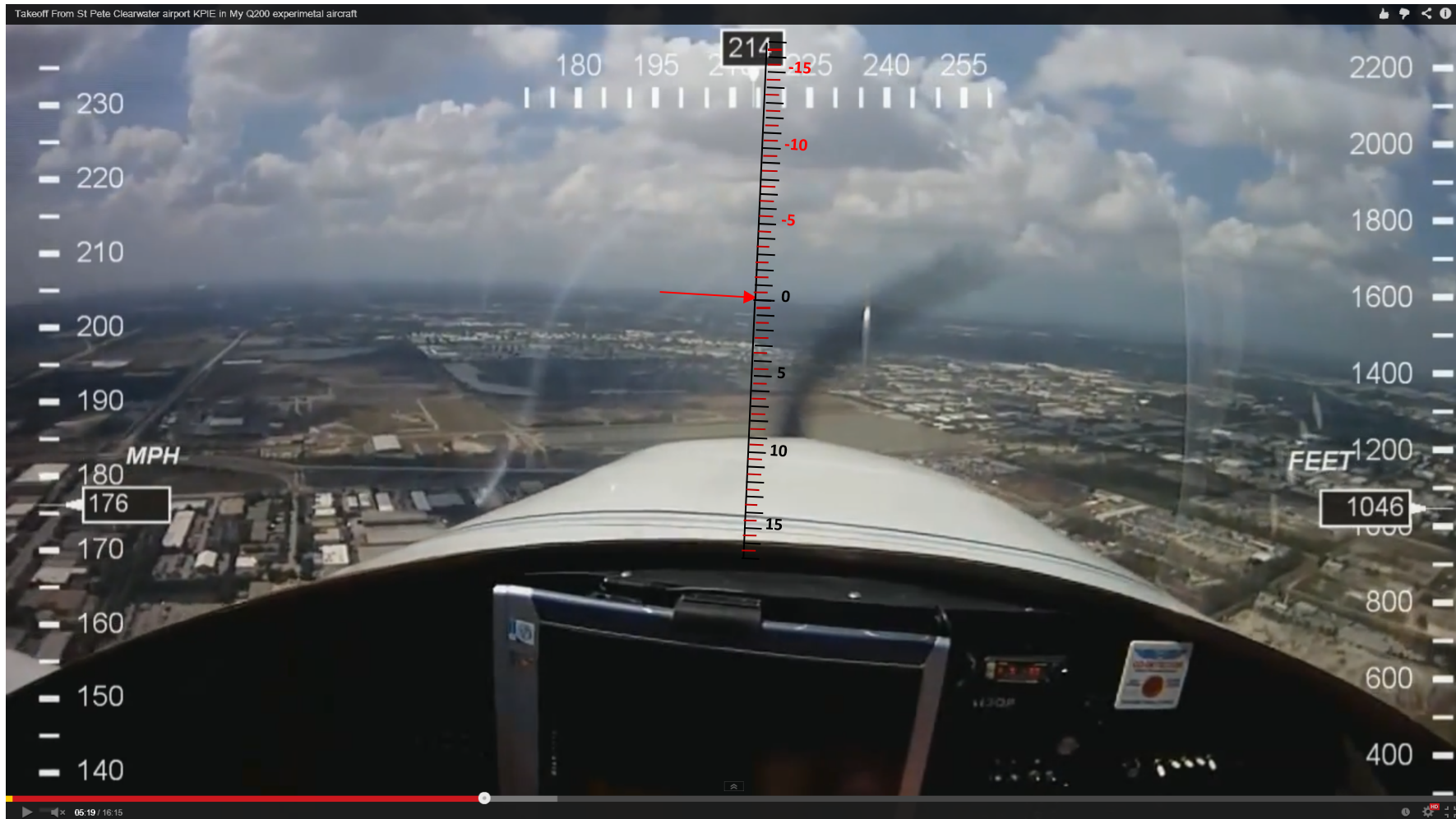
Figure 12. View from camera mounted on the seatback bulkhead. The vertical scale in the middle of the image is an angular scale that is calibrated to fixed points on the aircraft. The other scales (from Dashware) are: altitude (right), speed (left), and heading (top). This view is level, over 1000 feet MSL altitude and at max cruise (176 mph) at an alpha of -0.2 degrees. No confirmation of elevator deflection is possible at this point in flight.
