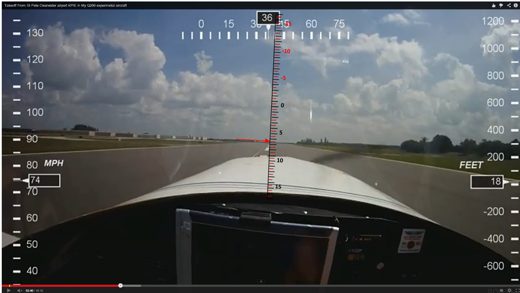
Figure 6. View from camera mounted on the seatback bulkhead. The vertical scale in the middle of the image is an angular scale that is calibrated to fixed points on the aircraft. The other scales (from Dashware) are: altitude (right), speed (left), and heading (top). This view is immediately after takeoff (74 mph) at an alpha of 6.5 degrees.
