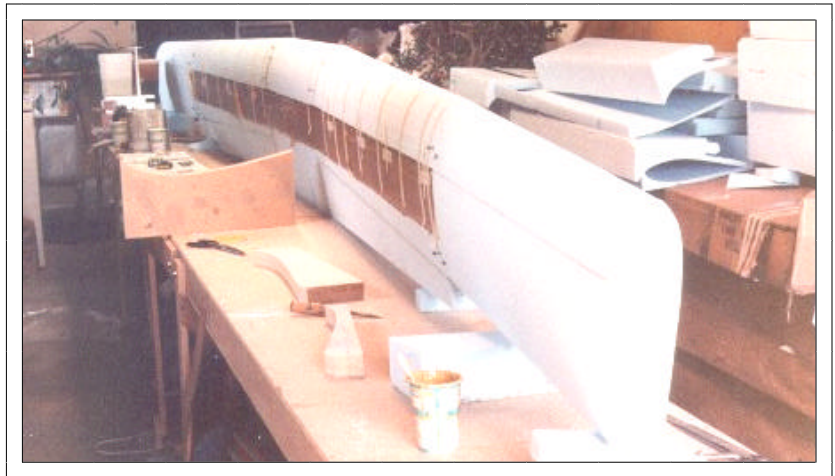
WING CORE WITH SHEAR WEB - note jig blocks for glassing.
