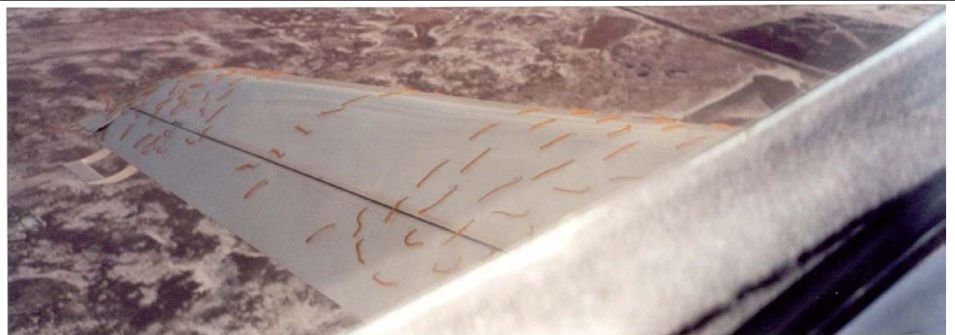
At 63 KTS, we see much more disturbance all across the airfoil, from about mid chord to the trailing edge. The elevator seems to be almost to the stop, judging by the gap at the tip.
