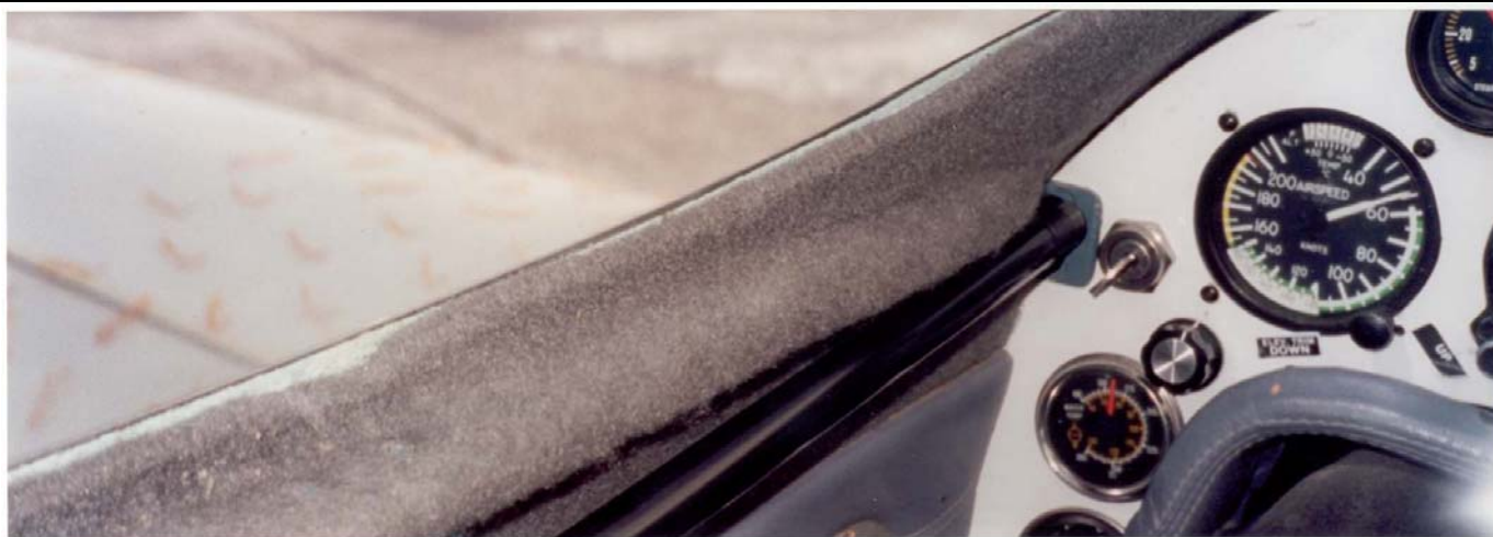
Ok, so I lied. The photo above is not the last in the series. Each shot of the canard that Reg took, he also shot a photo of the airspeed indicator. Problem was that he couldn't get both the yarns and the ASI in focus, in the same shot. In this photo, you can clearly see that the yarns are all over the place, and the airspeed is well below both the white and green arcs.
