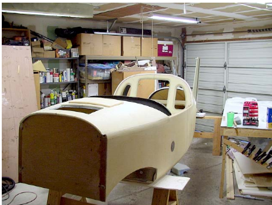
Tom's fuselage in his garage. It's not often that you get to see a fiberglass structure that still looks green, and hasn't turned brown yet. Note too the "roll" bar is more ingress and egress friendly, With the center "spoke" removed.
