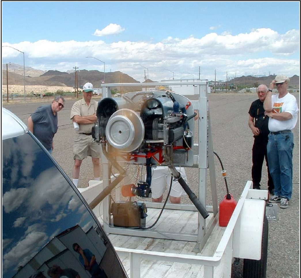
It took several tries to get the engine running just right. The carburetor being used has a typical automotive style choke, which unbeknownst to all, was partially closed during the initial runs. Once discovered and remedied, the engine ran just fine.
