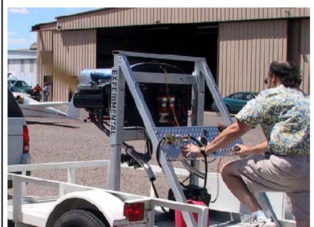
Pat runs the engine up to 2500 RPM with the mufflers removed.
