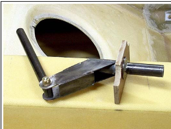
In DBFN issue #97, John Mason reported on a fix which significantly improves the aileron response by reinforcing the stick attachment fork. Here's Tom's adaptation of this same fix. You can see that Tom has welded plates to the forks, reinforcing the structure, making it a "box".
