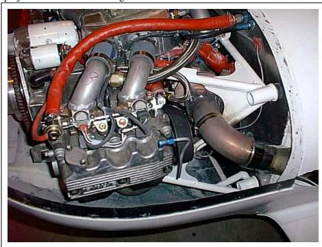
1998 Subaru EJ22, RHB5 turbo with an enhanced higher-capacity compressor section, for high altitude
