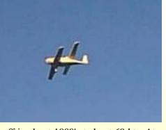
off in about 1000' at about 60 kts. At about 100 kts by the end of the runway. Climb out at approx 1500 ft/min. at 100-110 kts. Level at 4000' across the field throttled back with no boost indicating 145 kts. That engine was a pile of work but it sure is sweet to fly behind. Once I have more performance data I'll submit detail on it and the sooby 22. I'd like to say it was all worth it. Can't commit to going that far yet.
