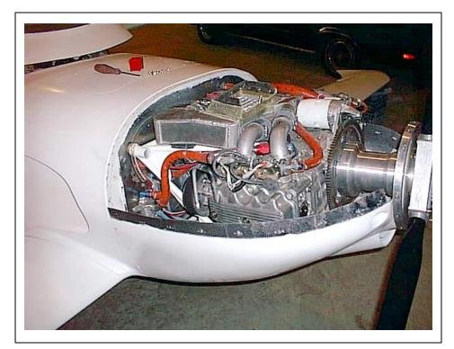
We removed all accessories, intake, and hoses, and the bell housing was cut off.
