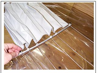
Upper left photo shows the business side of the center aluminum channel, which the bows ride upon. Double sided tape (shown orange) adheres the track to the canopy. The photo at the left shows the shade installed on one side of the rail and the wire ribs on the other. Mystery hand points to the thumb screw that locks the shade in the extend position. Van's has been flying the SunShade on their aircraft for some time now an seem to be pleased with the performance of the shade.
