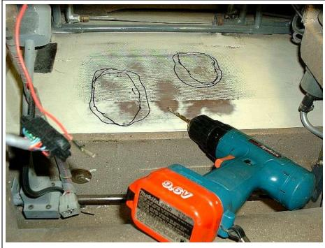
Paint removed, holes drilled, it's time to inject micro!
