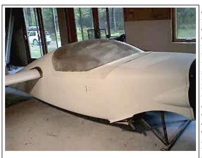
Right side, showing the canard root faring, and part of the "rolling fuselage" fixture.
