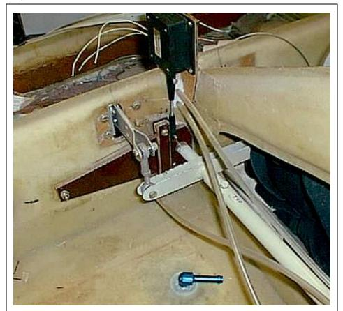
Check this photo closely. It's a very simple and elegant electrically actuated reflexor mechanism.
