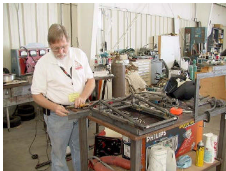
With the expert welding done by Terry Bailey, Paul Zimmerman crafted his Corvair engine mount from scratch. Paul attended William Wynne's "Corvair College" earlier this year, where he built his Corvair engine which will some day power his Dragonfly.
