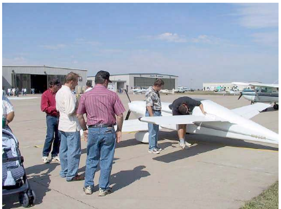
Drew measuring Terry O'Neil's wing incidence, with a group of interested onlookers. Using a digital level and a CAD template, he checked the incidence of every DF on the field.
