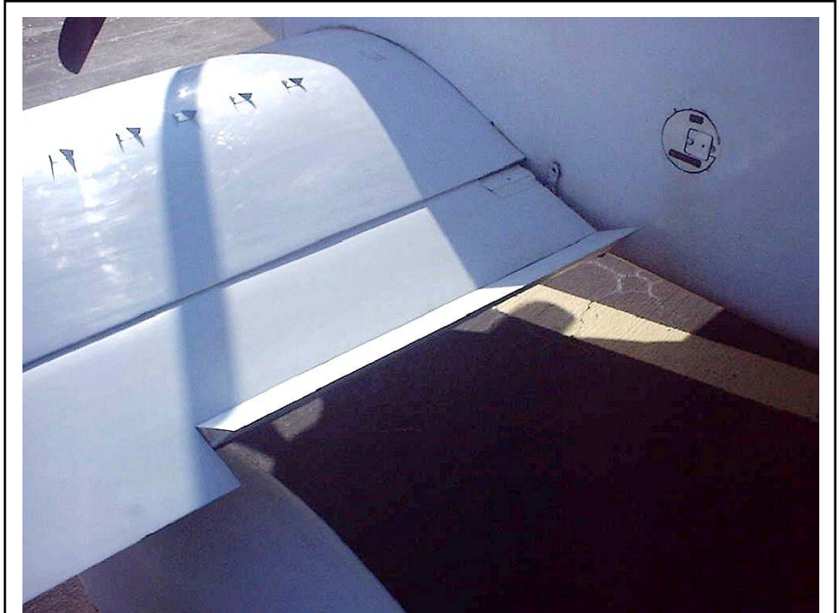
Tab in the full nose up trim, with the elevator in trail
