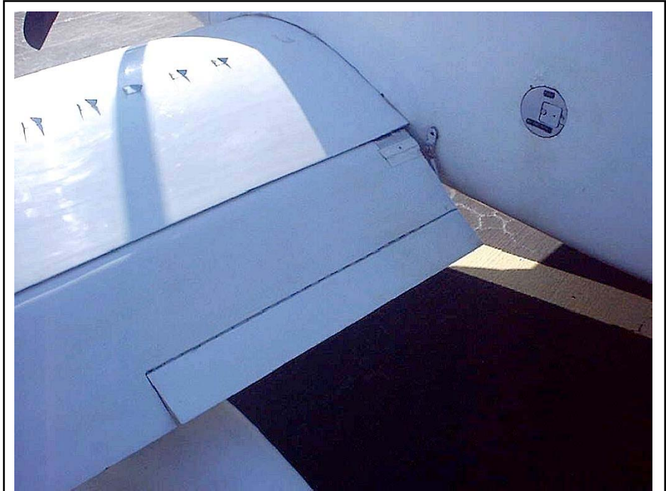
Terry's elevator tab replaces the sparrow strainer and the pitch trim mechanism. Additionally, the "anti-servo" function of this system adds stick loads in the pitch axis, helping to stabilize pitch, and to make stick pressures more equal, in the pitch and roll axis.
