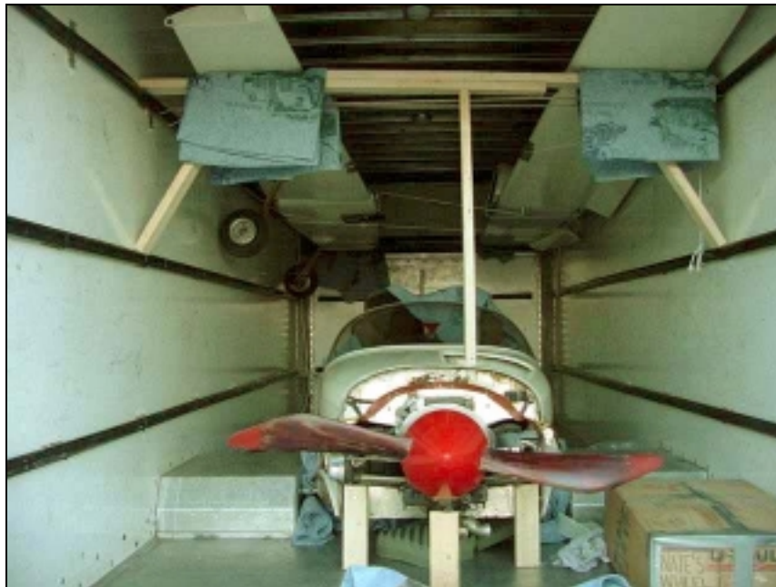
Finally nested in place. The engine is supported, the wings are suspended by the 2x4 truss, with safety rope added.
