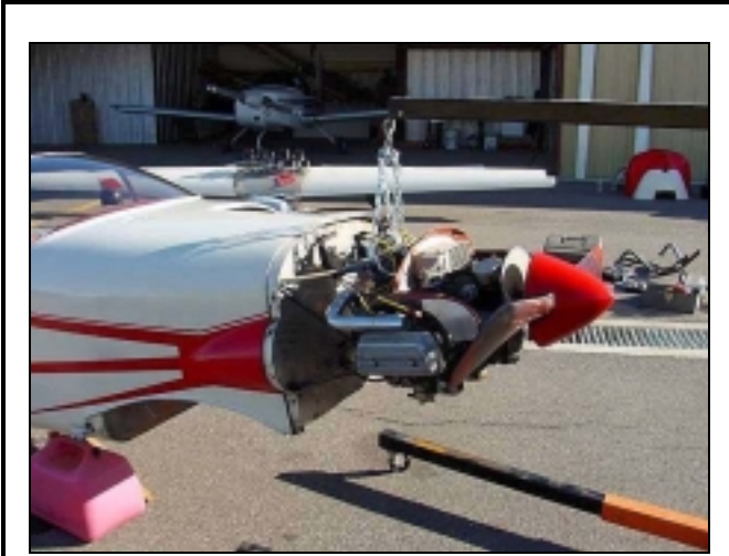
Engine hoist acted as a crane.
