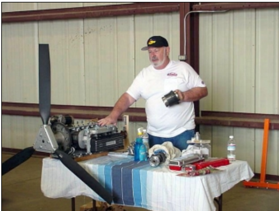
Bob Sutcliffe with John Moyle's 140hp 3100cc engine (custom built by Ted Hansen of Fresno CA) with Warp Drive propeller
